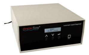
The Automatic Liquid Dispenser incorporates a pump and a flow-meter to deliver a measured volume of liquid. Delivery can be initiated at the press of a button, by external input signal, or automatically by means of an internal timer. The timer can be selected to start dispensing at regular intervals or start dispensing at set times of the day, on a daily or a weekly basis.
