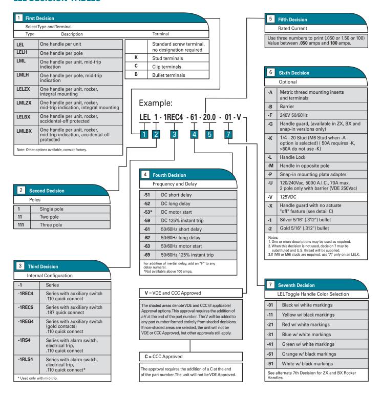
Notes: The LEL family of circuit breakers are designed to meet 8mm creepage and clearance requirements for installation Category 111, pollution degree 3, Case A as measured in IEC 664. Intended for use in equipment designed to comply with IEC 380, 435, 601 AND VDE 0730, 0804 & 0805.
