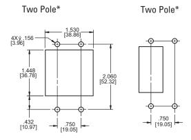
Panel Mounting Detail Tolerance ±.005 [.13] unless noted.
