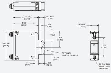
Note: Tolerance  $\pm$  .015 [.38] unless noted. Dimensions in brackets [ ] are millimeters.
