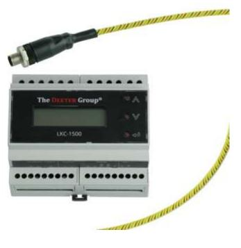
The LKC-1500 comprises a leak detector controller in a DIN-rail mounting enclosure and up to 1500m of leak sensing cable. The controller is able to detect a leak and indicate its position as a distance along the cable from the controller.
